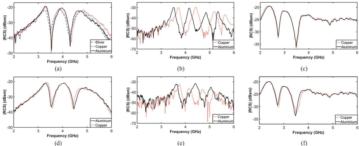
Figure 3:  $|\text{RCS}|$  Measurements results for (a) Circular tag on PET substrate, (b) Modified conical on PET substrate, (c) Dipole tag on PET substrate, (d) Circular tag on paper substrate, (e) Modified conical on paper substrate, and (f) Dipole tag on paper substrate.
