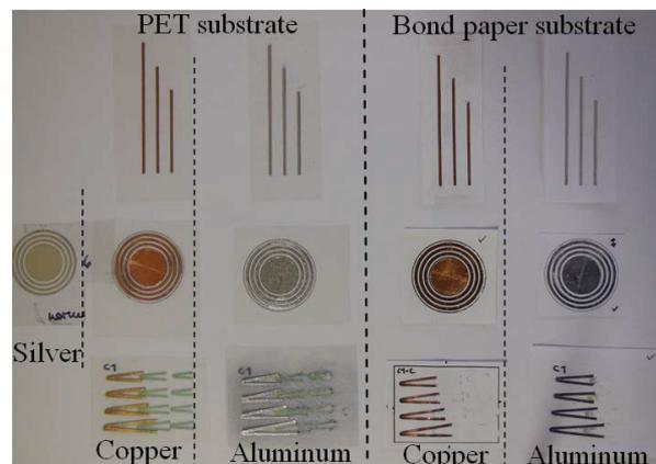
Figure 1: Fabricated UWB chipless tags using copper and aluminum tape on bond paper and PET, and single silver ink circular tag on PET.
