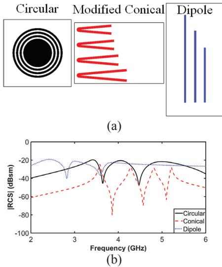
Figure 1: (a): Circular, modified conical and dipole like UWB chipless tags designs shape. (b) Simulated  $|RCS|$  based on copper strips for Circular tag, modified conical tag, and dipole tag.
